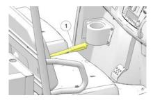
Always apply the service brakes before engaging or releasing the park brake.
