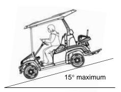
**WARNING!** Coasting down a hill could result in excessive speed, which could result in loss of control. Never travel down a hill at high speed.
