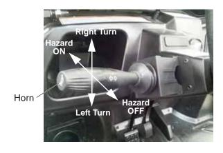
Move the turn signal lever downward to signal a left turn. The left turn signal lamp below the front headlight will flash. The left turn indicator on the dash will also flash.
