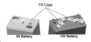
3. Maintain the fluid level between the battery plates and the bottom of the fill well. Add distilled water as needed. Do not overfill. Reinstall the fill well cap securely.
