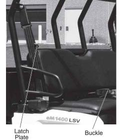
5. To release the seat belt, press the square red button in the buckle's center. If necessary, slide the buckle down the webbing to allow it to retract fully.
