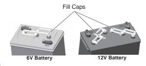
3. Maintain the fluid level between the battery plates and the bottom of the fill well. Add distilled water as needed. Do not overfill. Reinstall the fill well cap securely.
