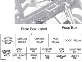
Open the hood to access the fuse box. See the label attached to the fuse box cover for the function and amp rating of each fuse. The spare and heater coil fuses are used for accessories.
