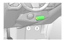
When the park brake is set and the brake indicator is illuminated, the vehicle will not move.
