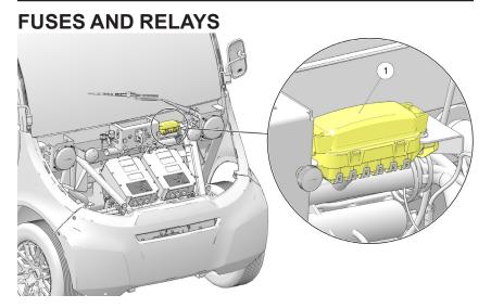
If you experience electrical failures not related to the batteries, a fuse may need replacement. Locate and correct any short circuits that may have caused the blown fuse, then replace the fuse. If you suspect a relay or diode needs replacement, your authorized GEM dealer can assist.
