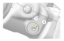
Leaving the key in the ON position will discharge the batteries. Always turn the key to the OFF position when not operating. Remove the key from the ignition to prevent unauthorized use.
