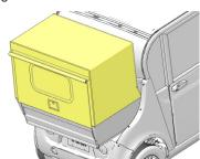
Never carry a passenger on a rear accessory back. Do not overload an accessory back. Overloading the vehicle can reduce stability and handling and could cause loss of control. *Never exceed the GVWR or the GAWR of the vehicle.* See page 17.
